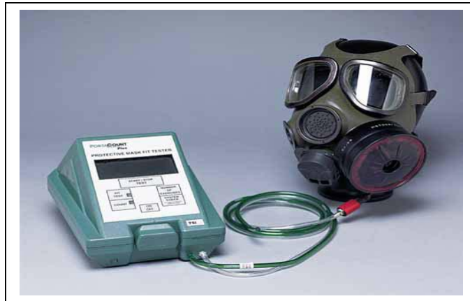
Figure A-6. M41 Protection Assessment Test System
